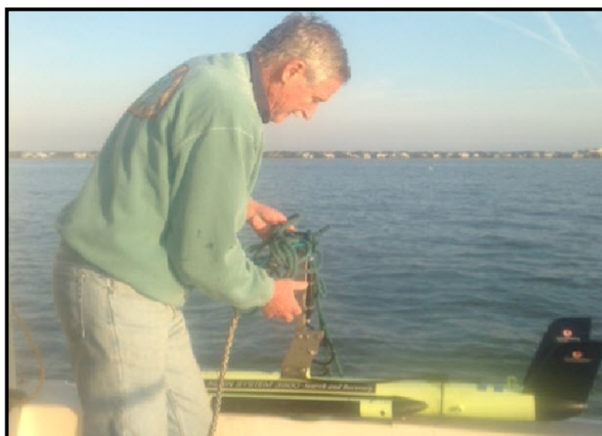
Figure 6. KLEIN SYSTEM 3900 digital sidescan sonar.
