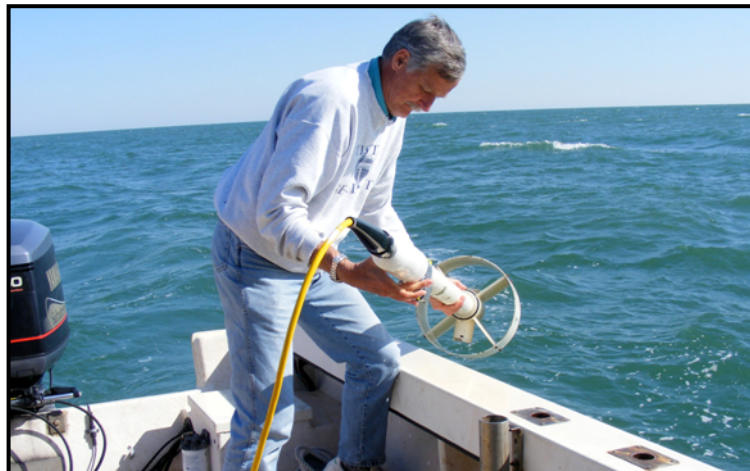
Figure 5. GEOMETRICS G-881 cesium vapor magnetometer.
